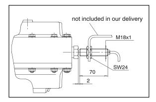
Retrofitting of the EOC system in already installed FLUDEX couplings is possible without reworking in the case of sizes 297-755.
