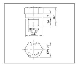
The transmitter comprises an AL bearer screw with an in-built magnet /system which changes its field strength according to the temperature. The magnet system is designed so that at a pick-up distance of 2 mm a cut-out temperature of 125 °C results. If the gap between the pick-up and the transmitter is greater, the EOC system switches at lower temperatures.
