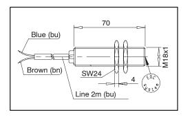
The pick-up records the magnetic field of the transmitter each time it is passed and, if there is sufficient field strength, sends a square-wave signal to the evaluating instrument. Below a fixed field-strength threshold (temperature switching point) no signal is sent.
